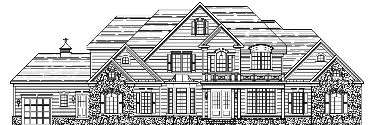
FRONT ELEVATION ELEVATION #3B W/ SIDING & STONE
