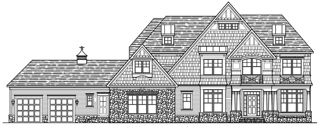
FRONT ELEVATION ELEVATION #9B 04-27-2023 W/ SIDING & STONE W/ MULTI GEN. 4-CAR GARAGE
