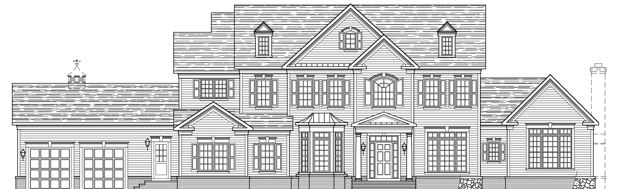
FRONT ELEVATION * ELEVATION #8A W/ FRONT LOAD 2-CAR GARAGE W/ CLUB ROOM STONE IS OPTIONAL 06-09-22
