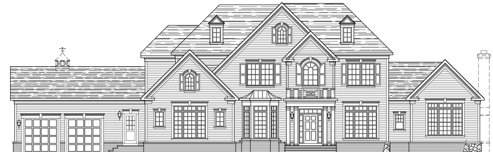
FRONT ELEVATION * ELEVATION #13A W/ FRONT LOAD 2-CAR GARAGE W/ CLUB ROOM STONE IS OPTIONAL 06-09-22
