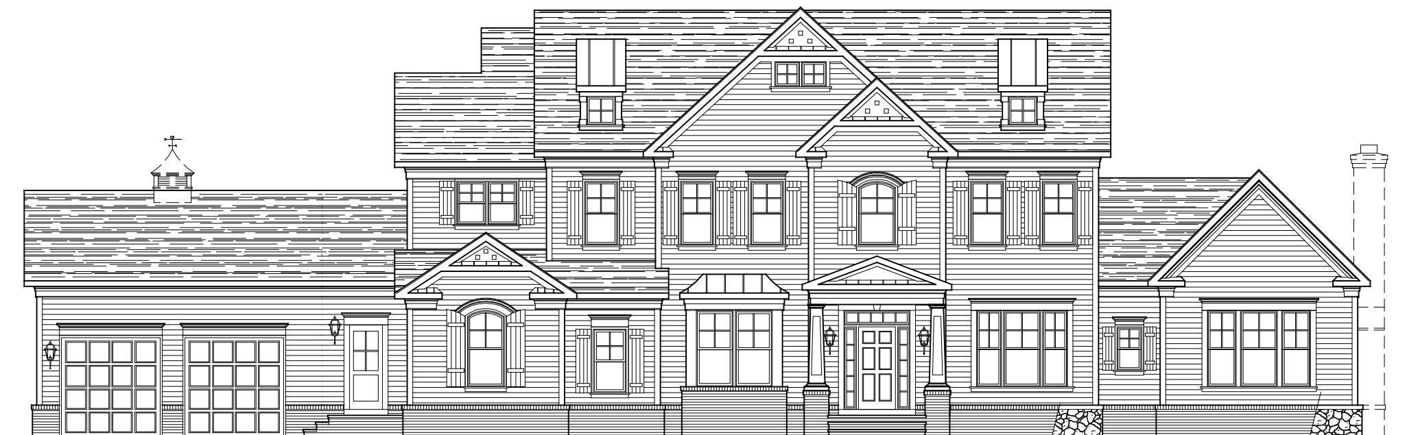
FRONT ELEVATION * ELEVATION #4A W/ FRONT LOAD 2-CAR GARAGE W/ CLUB ROOM STONE IS OPTIONAL 06-09-22
