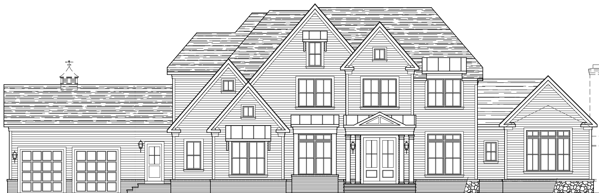
FRONT ELEVATION * ELEVATION #16A W/ FRONT LOAD 2-CAR GARAGE W/ CLUB ROOM STONE IS OPTIONAL 06-09-22
