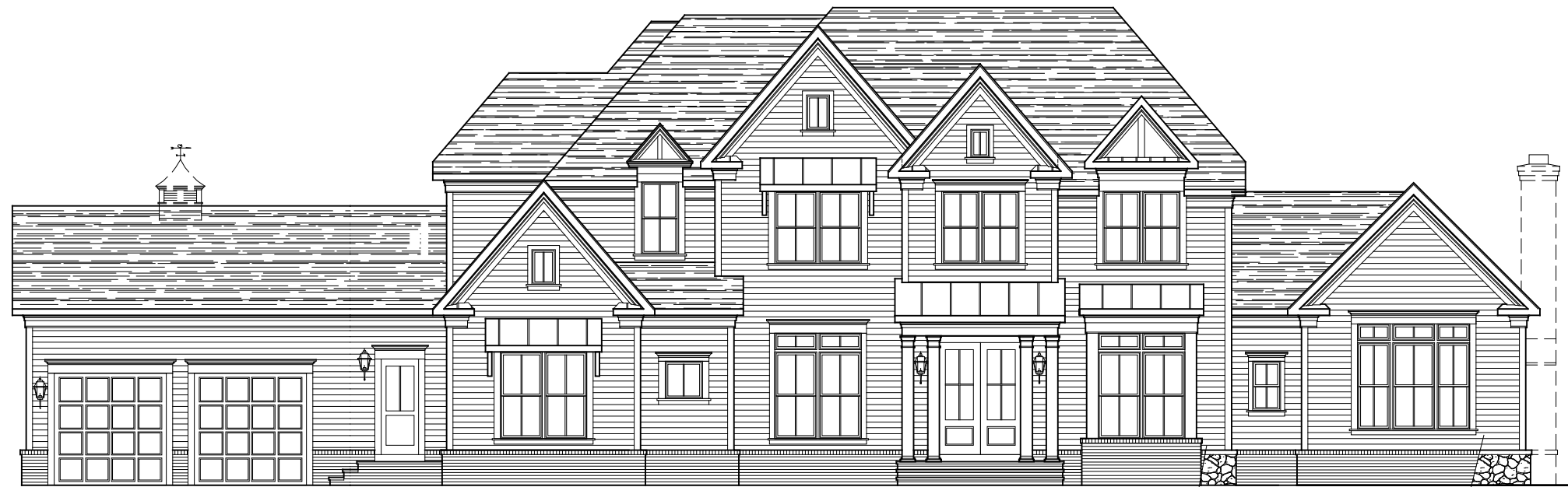
FRONT ELEVATION * ELEVATION #15A W/ FRONT LOAD 2-CAR GARAGE W/ CLUB ROOM STONE IS OPTIONAL 06-09-22
