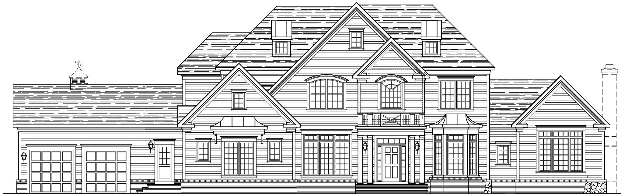
FRONT ELEVATION * ELEVATION #11A W/ FRONT LOAD 2-CAR GARAGE W/ CLUB ROOM STONE IS OPTIONAL 06-09-22
