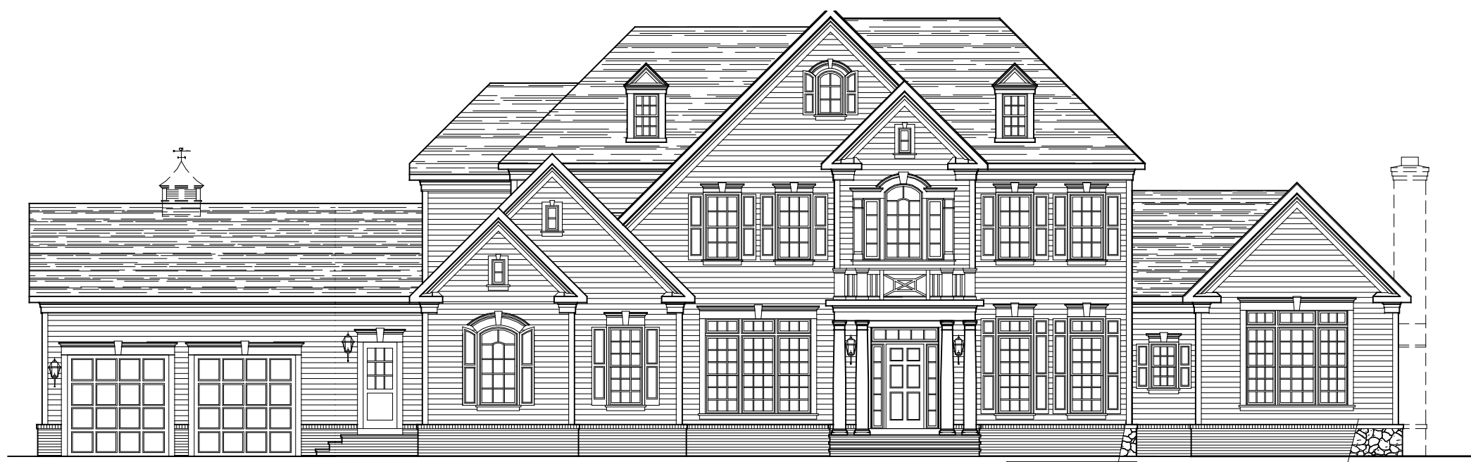
FRONT ELEVATION * ELEVATION #9A W/ FRONT LOAD 2-CAR GARAGE W/ CLUB ROOM STONE IS OPTIONAL 06-09-22
