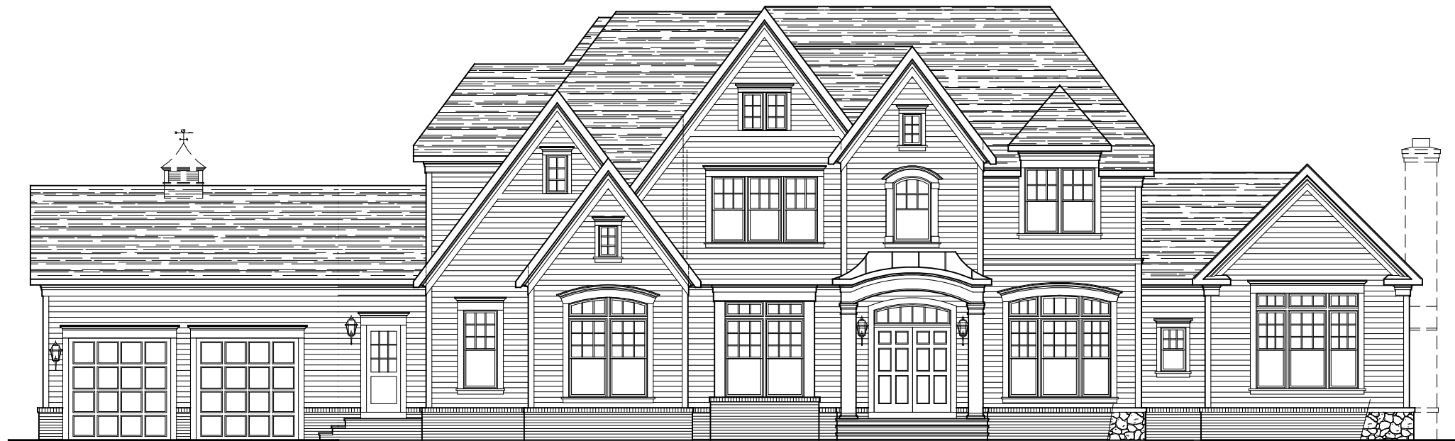
FRONT ELEVATION * ELEVATION #12A W/ FRONT LOAD 2-CAR GARAGE W/ CLUB ROOM STONE IS OPTIONAL 06-09-22
