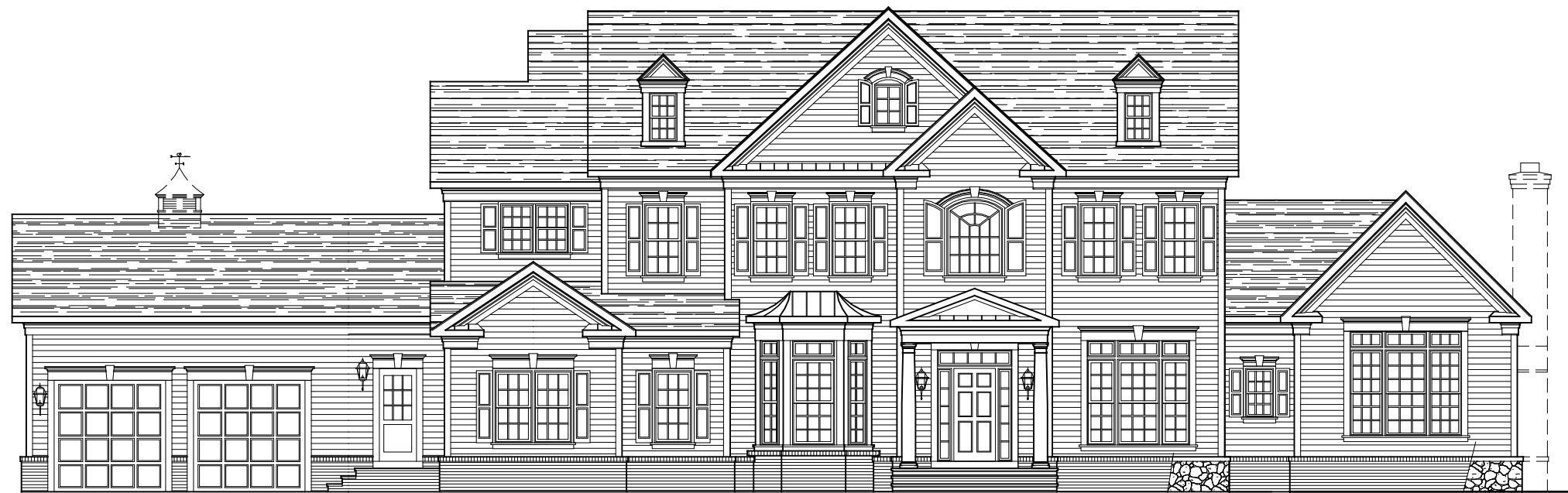
FRONT ELEVATION * ELEVATION #6A W/ FRONT LOAD 2-CAR GARAGE W/ CLUB ROOM STONE IS OPTIONAL 08-18-22
