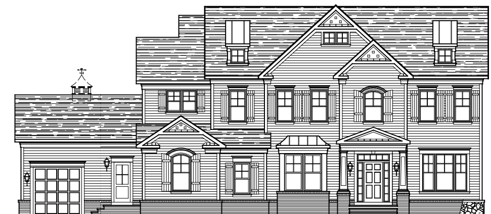
FRONT ELEVATION * ELEVATION #4A W/ FRONT LOAD 1-CAR GARAGE STONE IS OPTIONAL 08-18-22
