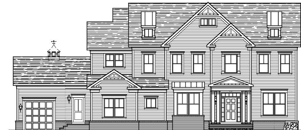
FRONT ELEVATION * ELEVATION #5A W/ FRONT LOAD 1-CAR GARAGE STONE IS OPTIONAL 08-18-22
