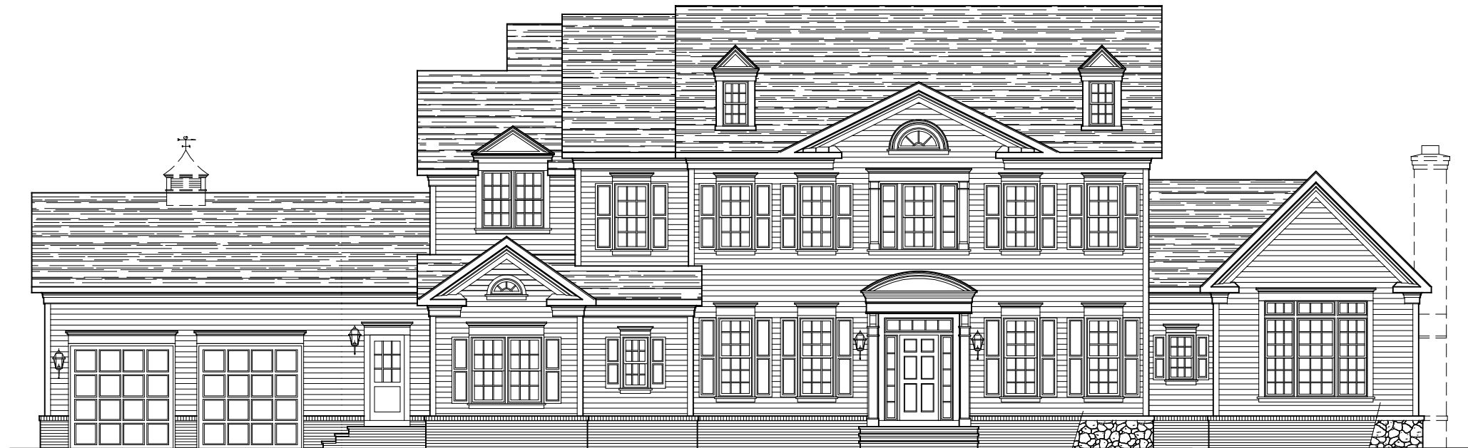
FRONT ELEVATION * ELEVATION #2A W/ FRONT LOAD 2-CAR GARAGE W/ CLUB ROOM 08-18-22 STONE IS OPTIONAL
