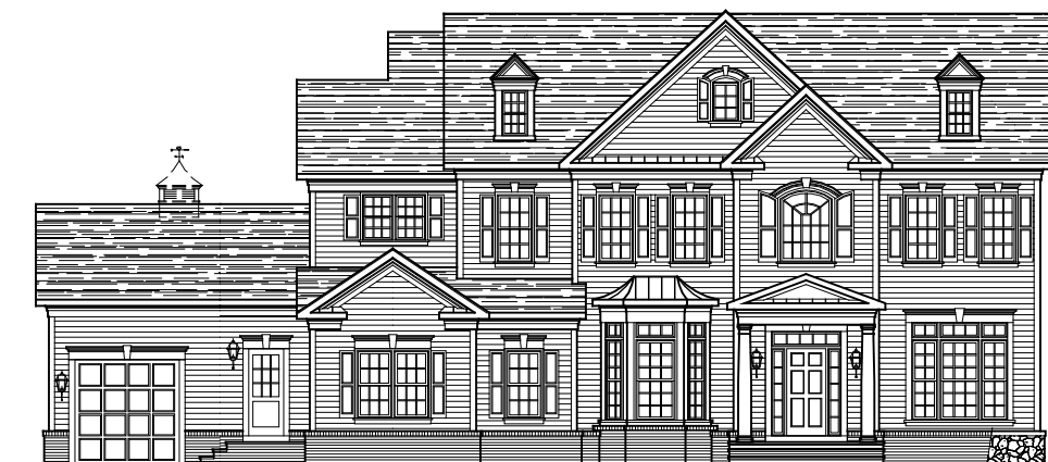
FRONT ELEVATION * ELEVATION #6A W/ FRONT LOAD 1-CAR GARAGE STONE IS OPTIONAL 08-18-22
