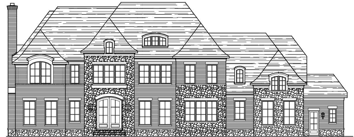
* SHOWN W/ OPT. STONE WATER TABLE * SHOWN W/ OPT. STONE ACCENTS FRONT ELEVATION ELEVATION 10A W/ BRICK & STONE 05-19-23 STONE IS OPTIONAL
