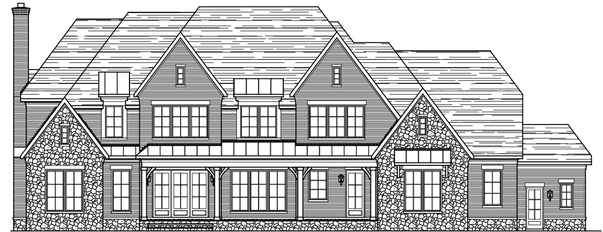
* SHOWN W/ OPT. STONE WATER TABLE * SHOWN W/ OPT. STONE ACCENTS FRONT ELEVATION ELEVATION 4B W/ BRICK & STONE 05-19-23 STONE IS OPTIONAL
