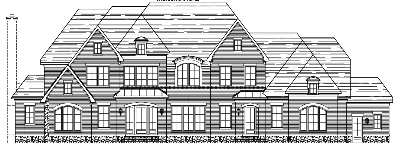
* SHOWN W/ OPT. STONE WATER TABLE * SHOWN W/ OPT. REAR CLUB ROOM FRONT ELEVATION ELEVATION 9A W/ STANDARD FULL BRICK W/ STONE BASE 05-19-23 STONE IS OPTIONAL
