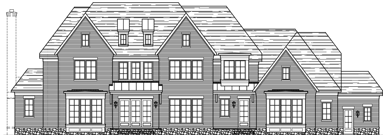
* SHOWN W/ OPT. STONE WATER TABLE * SHOWN W/ OPT. REAR CLUB ROOM FRONT ELEVATION ELEVATION 3A W/ STANDARD FULL BRICK W/ STONE BASE 05-19-23 STONE IS OPTIONAL
