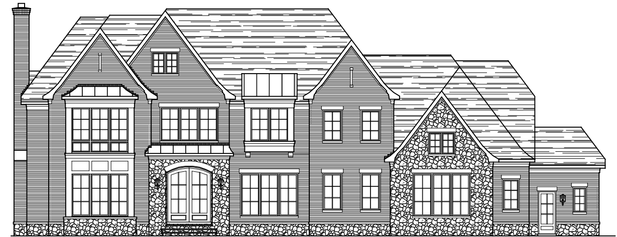
* SHOWN W/ OPT. STONE WATER TABLE * SHOWN W/ OPT. STONE ACCENTS FRONT ELEVATION ELEVATION 8A W/ BRICK & STONE 05-19-23 STONE IS OPTIONAL
