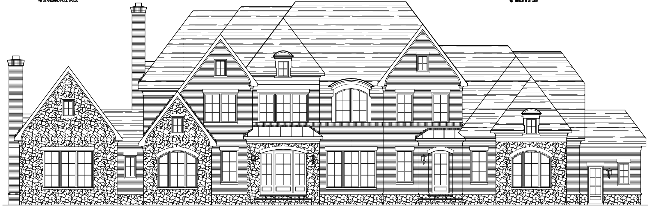
* SHOWN W/ OPT. STONE WATER TABLE * SHOWN W/ OPT. STONE ACCENTS * SHOWN W/ OPT. SIDE CLUB ROOM FRONT ELEVATION ELEVATION 9A W/ BRICK & STONE 05-19-23 STONE IS OPTIONAL
