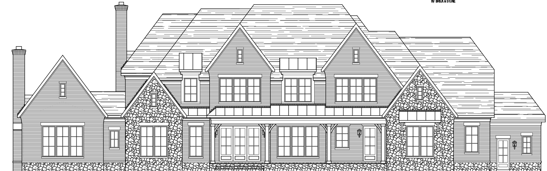
* SHOWN W/ OPT. STONE WATER TABLE * SHOWN W/ OPT. STONE ACCENTS * SHOWN W/ OPT. SIDE CLUB ROOM FRONT ELEVATION ELEVATION 4B W/ BRICK & STONE 05-19-23 STONE IS OPTIONAL
