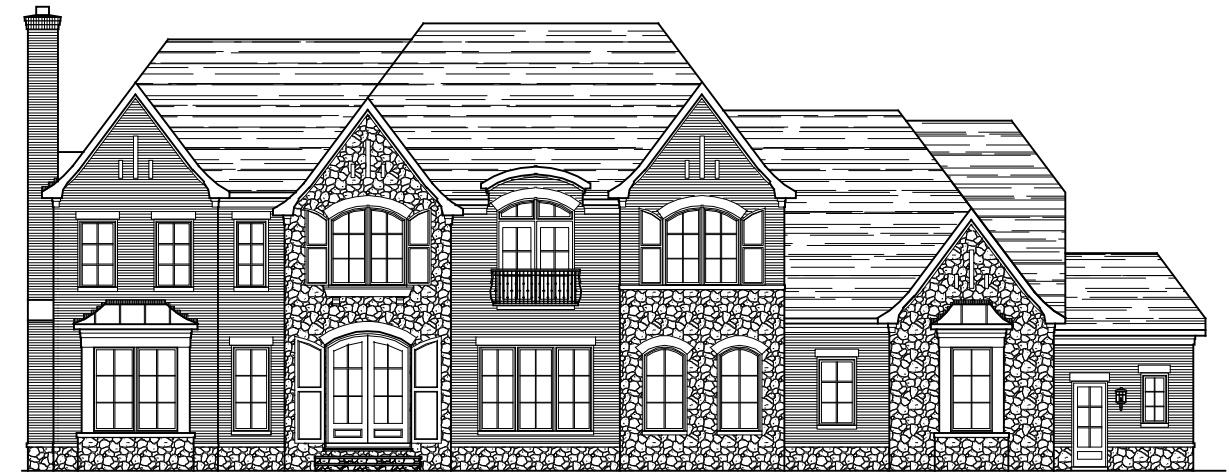
* SHOWN W/ OPT. STONE WATER TABLE * SHOWN W/ OPT. STONE ACCENTS FRONT ELEVATION ELEVATION 11A W/ BRICK & STONE 05-19-23 STONE IS OPTIONAL
