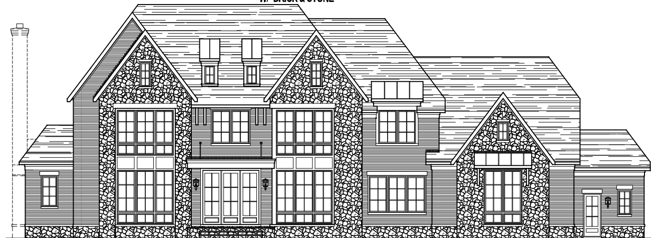
* SHOWN W/ OPT. STONE WATER TABLE * SHOWN W/ OPT. REAR CLUB ROOM FRONT ELEVATION ELEVATION 12A W/ BRICK & STONE 05-19-23 STONE IS OPTIONAL
