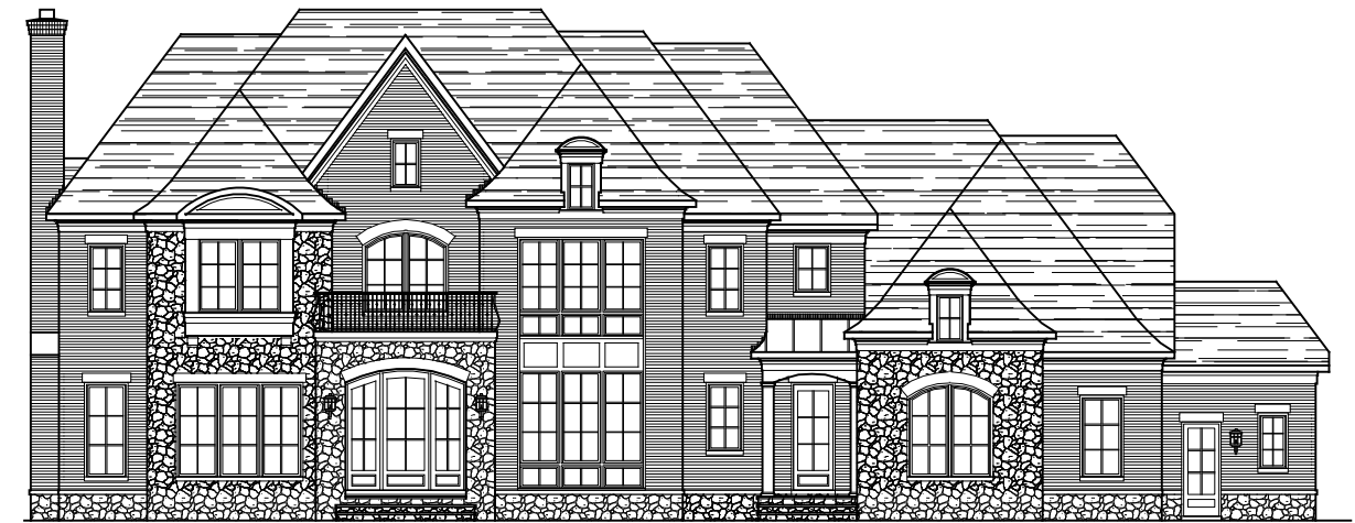
* SHOWN W/ OPT. STONE WATER TABLE * SHOWN W/ OPT. STONE ACCENTS FRONT ELEVATION ELEVATION 6A W/ BRICK & STONE 05-19-23 STONE IS OPTIONAL
