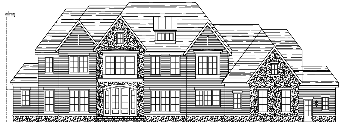
* SHOWN W/ OPT. STONE WATER TABLE * SHOWN W/ OPT. STONE ACCENTS * SHOWN W/ OPT. SIDE CLUB ROOM FRONT ELEVATION ELEVATION 5A W/ BRICK & STONE 05-19-23 STONE IS OPTIONAL
