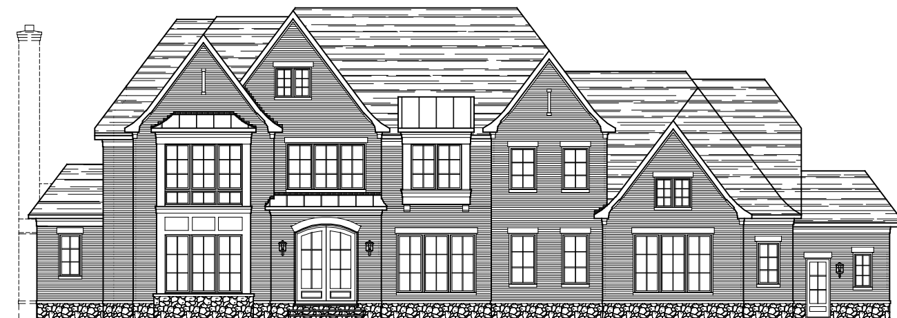
* SHOWN W/ OPT. STONE WATER TABLE * SHOWN W/ OPT. REAR CLUB ROOM FRONT ELEVATION ELEVATION 8A W/ STANDARD FULL BRICK W/ STONE BASE 05-19-23 STONE IS OPTIONAL
