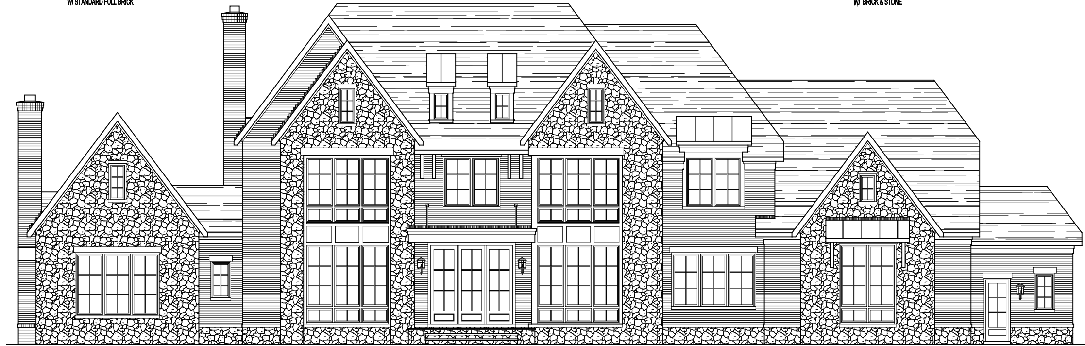
* SHOWN W/ OPT. STONE WATER TABLE * SHOWN W/ OPT. REAR CLUB ROOM FRONT ELEVATION ELEVATION 12A W/ BRICK & STONE 05-19-23 STONE IS OPTIONAL
