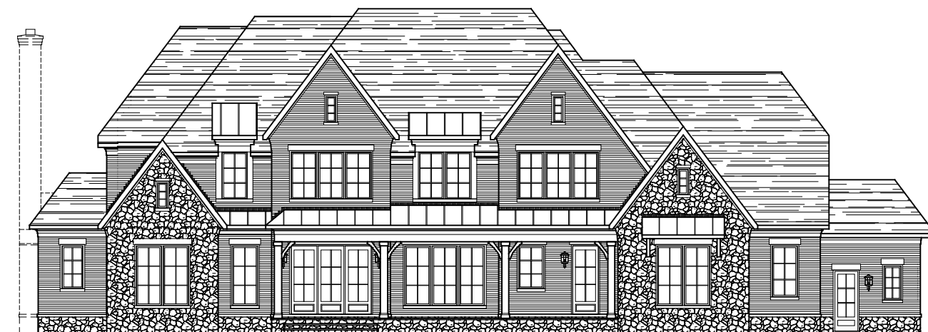
* SHOWN W/ OPT. STONE WATER TABLE * SHOWN W/ OPT. REAR CLUB ROOM FRONT ELEVATION ELEVATION 4B W/ BRICK & STONE 05-19-23 STONE IS OPTIONAL
