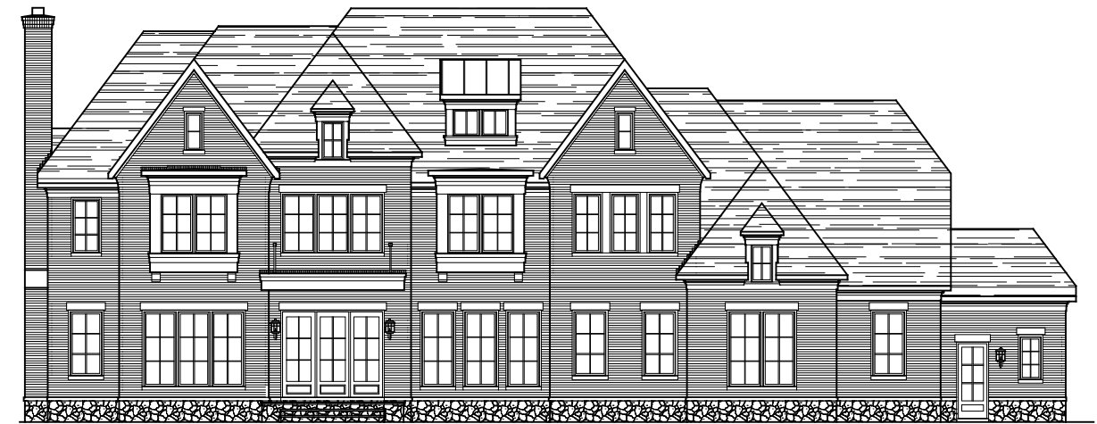
* SHOWN W/ OPT. STONE WATER TABLE FRONT ELEVATION ELEVATION 3A W/ BRICK & STONE 05-19-23 STONE IS OPTIONAL
