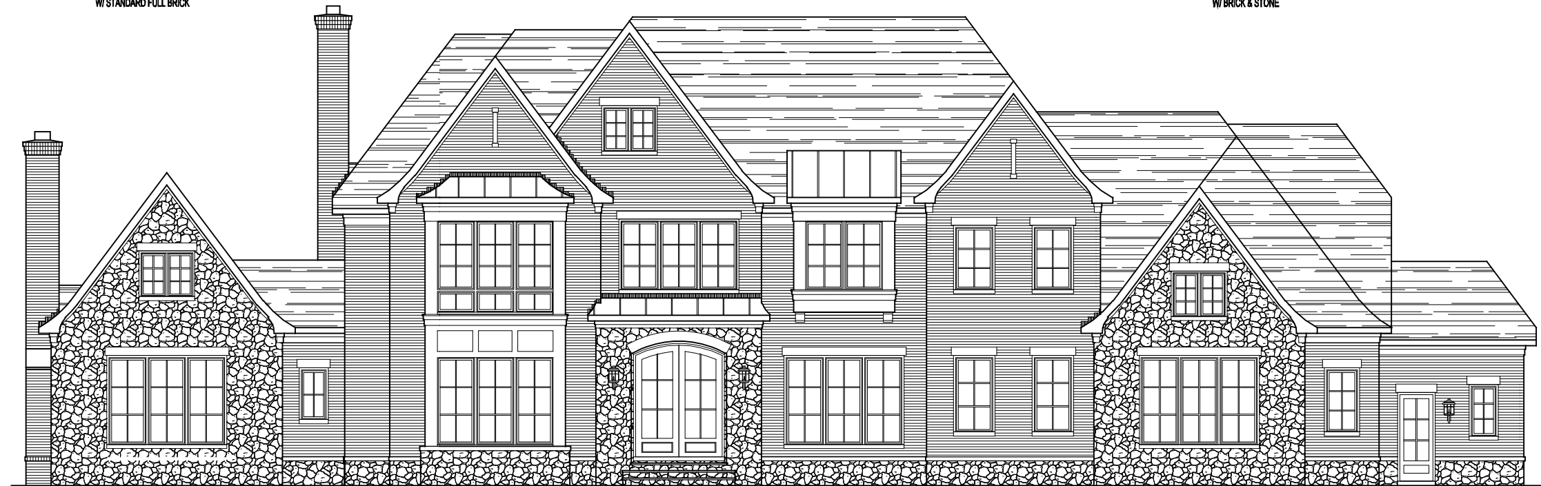
* SHOWN W/ OPT. STONE WATER TABLE * SHOWN W/ OPT. STONE ACCENTS * SHOWN W/ OPT. SIDE CLUB ROOM FRONT ELEVATION ELEVATION 8A W/ BRICK & STONE 05-19-23 STONE IS OPTIONAL
