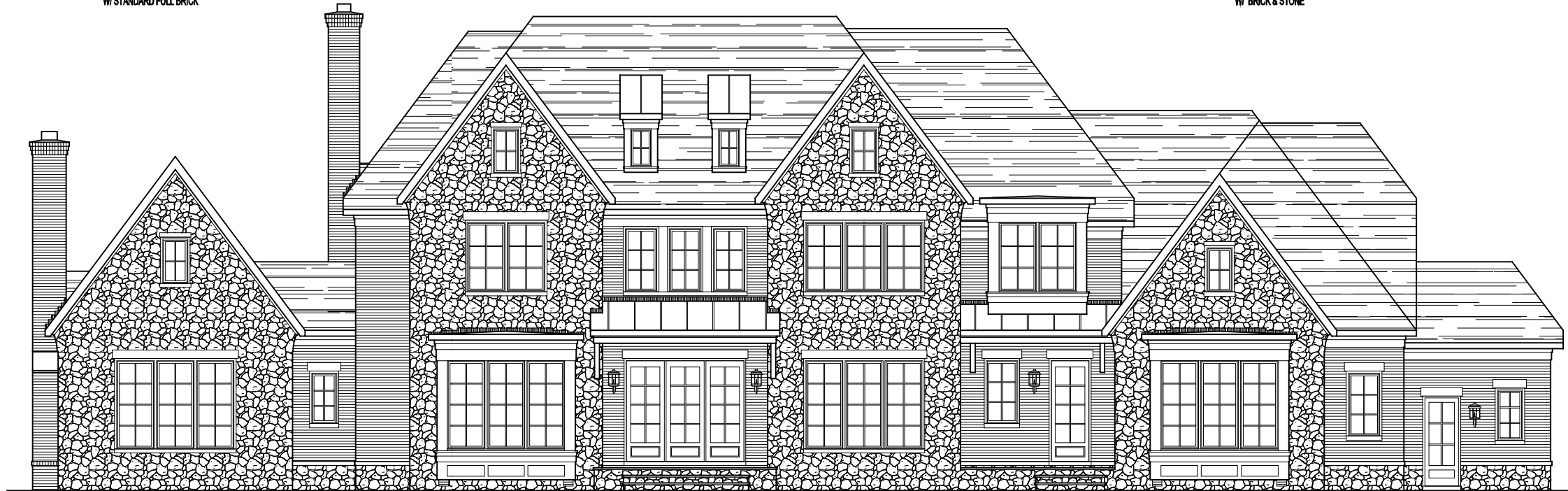
* SHOWN W/ OPT. STONE WATER TABLE * SHOWN W/ OPT. STONE ACCENTS * SHOWN W/ OPT. SIDE CLUB ROOM FRONT ELEVATION ELEVATION 3A W/ BRICK & STONE 05-19-23 STONE IS OPTIONAL
