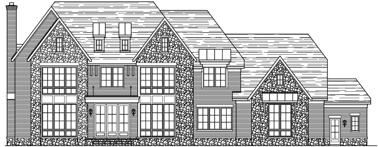
* SHOWN W/ OPT. STONE WATER TABLE * SHOWN W/ OPT. STONE ACCENTS FRONT ELEVATION ELEVATION 12A W/ BRICK & STONE 05-19-23 STONE IS OPTIONAL
