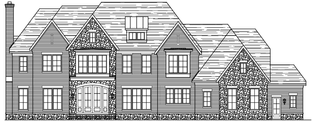
* SHOWN W/ OPT. STONE WATER TABLE * SHOWN W/ OPT. STONE ACCENTS FRONT ELEVATION ELEVATION 5A W/ BRICK & STONE 05-19-23 STONE IS OPTIONAL
