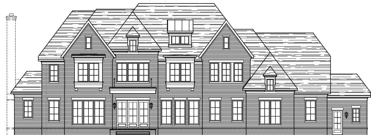
* SHOWN W/ OPT. REAR CLUB ROOM FRONT ELEVATION ELEVATION 2A W/ STANDARD FULL BRICK 05-19-23
