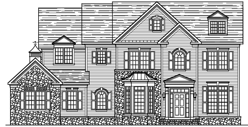
FRONT ELEVATION ELEVATION #4 W/ STONE AND SIDING
