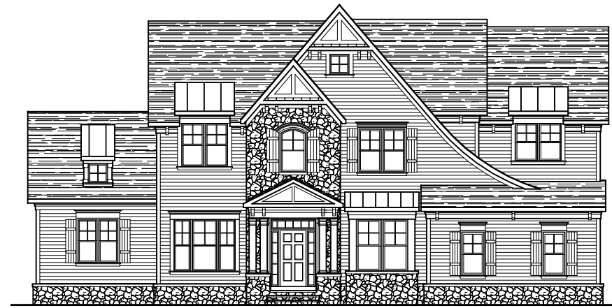
FRONT ELEVATION ELEVATION #7A W/ SIDING AND STONE FRONT 02-04-22 STONE IS OPTIONAL
