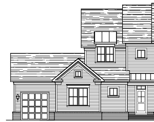
FRONT ELEVATION ELEVATION #9B W/ MUDROOM DOOR 07-16-21
