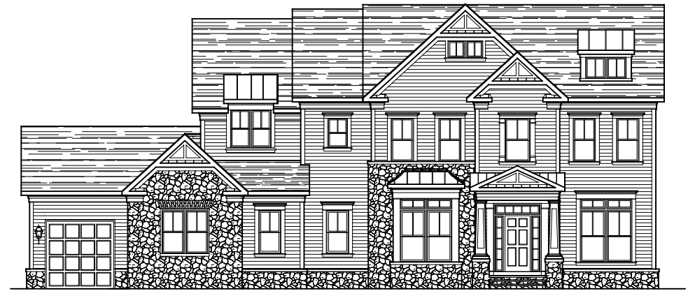
FRONT ELEVATION ELEVATION #5A W/ STONE AND SIDING 07-16-21
